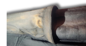
Soot/ Scorch marks
